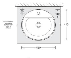
MAY BE SEALED TO TER TOP USING ACETIC CURE INE SEALANT OT USE EPOXY ADHESIVES
