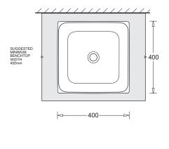
NOTE: BASIN MAY BE SEALED TO COUNTER TOP USING ACETIC CURE SILICONE SEALANT DO NOT USE EPOXY ADHESIVES
