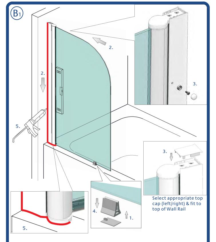
1. Push support & basepad onto bottom edge of glass toward outer end of screen.
