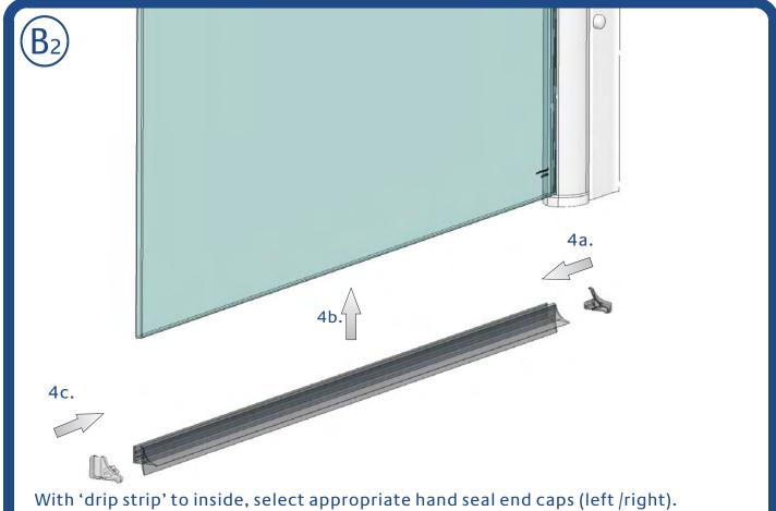
4a. Apply clear silicone sealant to hinge end cap & push into seal.
