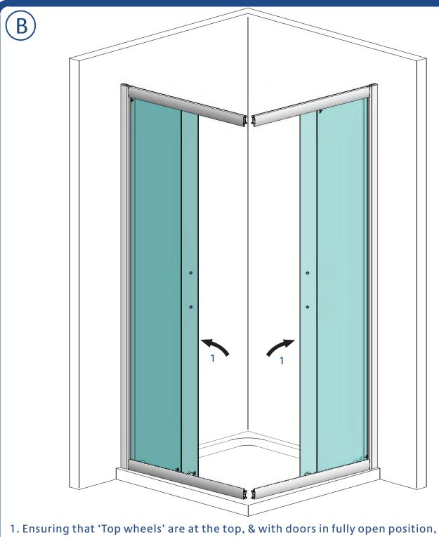
carefully lift panel sub assemblies onto tray & push fully into wall profiles.
