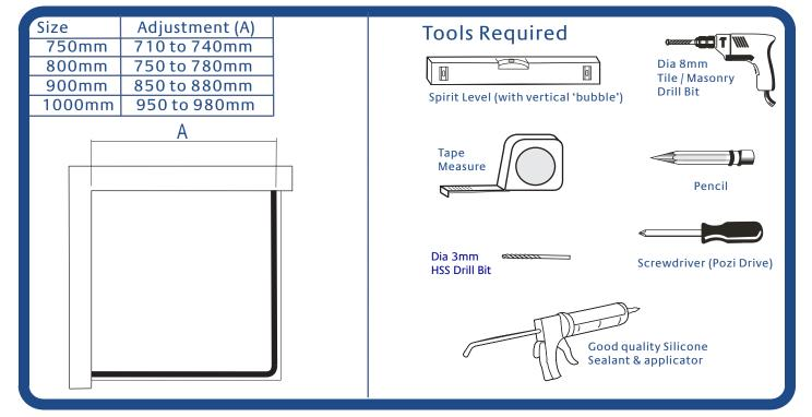
Ensure tray is correctly levelled & that tray / wall (tile) joints are sealed & cured over entire length of tray sides (See Fig A) prior to fitting enclosure.
