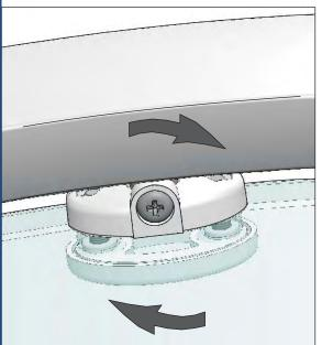
Adjust door heights until doors run smoothly on rails. Adjust door angles so that magnetic seals meet squarely & hold doors in closed position. Turn adjusting screw clockwise to raise door.
