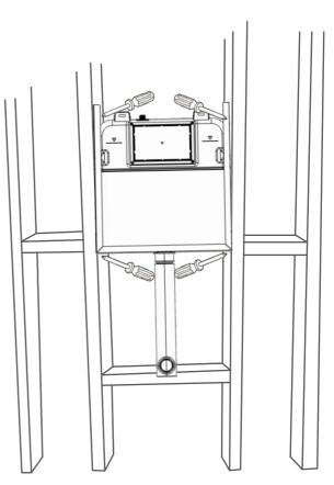
Note: Use mounting bracket as a template to locate hole positions
