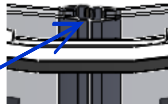
Fit magnetic seal to leading edge of door.
